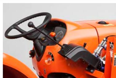
The loader valve and joystick comes standard with either loader package. The joystick is ergonomically placed within easy reach of the operator.
